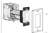
Use the provided screws to secure the light switch to the electrical box. Then, replace the wall plate.
